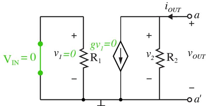
Turn off the independent voltage source such that  $V_{IN} = v_1 = 0$ .
