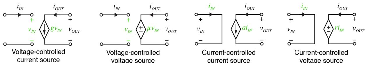
Circuits including dependent sources can be analyzed using the Nodal analysis, Intuitive, Thévenin/Norton, and Superposition methods. Here we will go through some example circuits with dependent sources.
