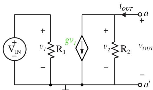
Note that this circuit has a voltage-controlled current source.
