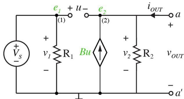
To find the **Thévenin equivalent** for this circuit, we need to find  $V_{TH}$  and  $R_{TH}$ .
