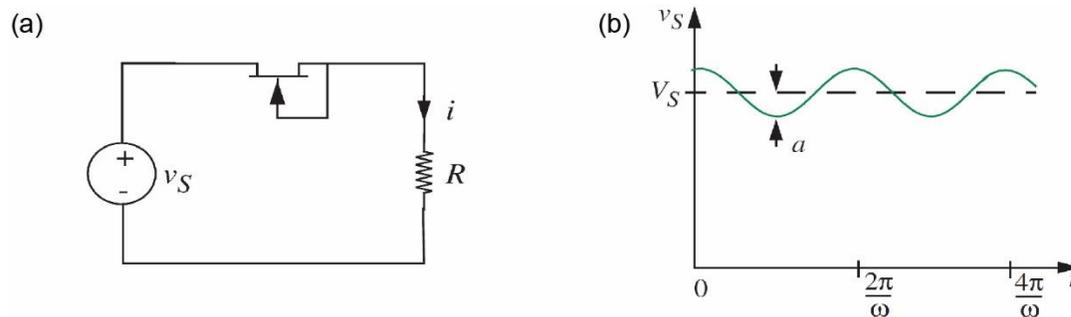
We are interested in building a regulated current source. That is, even if there is a small noise (oscillation) in the driving voltage, the output current  $i$  will have no oscillation. Let us consider the circuit shown above (a). First, we use KVL to solve for the large signal behavior:
