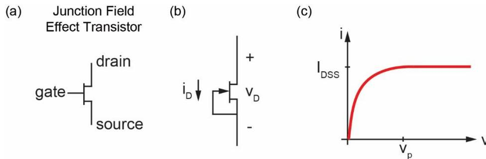
The device physics show this component has a “pinch-off” voltage  $v_p$ . The i-v characteristic is given by:
