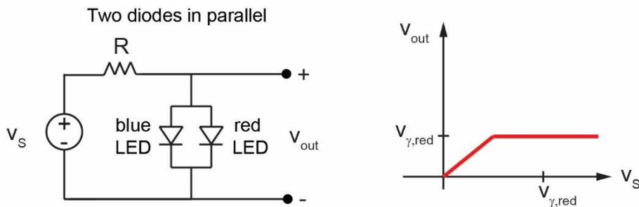
It also has two possibilities. If  $V_S < v_{\gamma,red}$ , then both LEDs will be off. If  $V_S > v_{\gamma,red}$ , then the red LED will turn on. However, because  $v_{\gamma,red} < v_{\gamma,blue}$ , the blue LED will never turn on. In practice, we rarely put LEDs in parallel without adding resistors in series.
