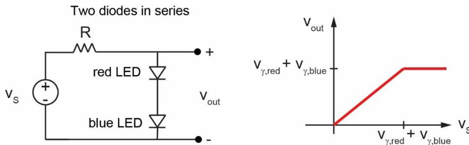
There are two possibilities. If  $V_s > v_{\gamma,red} + v_{\gamma,blue} = 4.7\text{ V}$ , then both diodes will turn on (both switches will be closed). In contrast, if  $V_s < v_{\gamma,red} + v_{\gamma,blue}$ , then BOTH diodes will turn off (both switches will be open). The voltage across the diodes will distribute in such a way that none will
