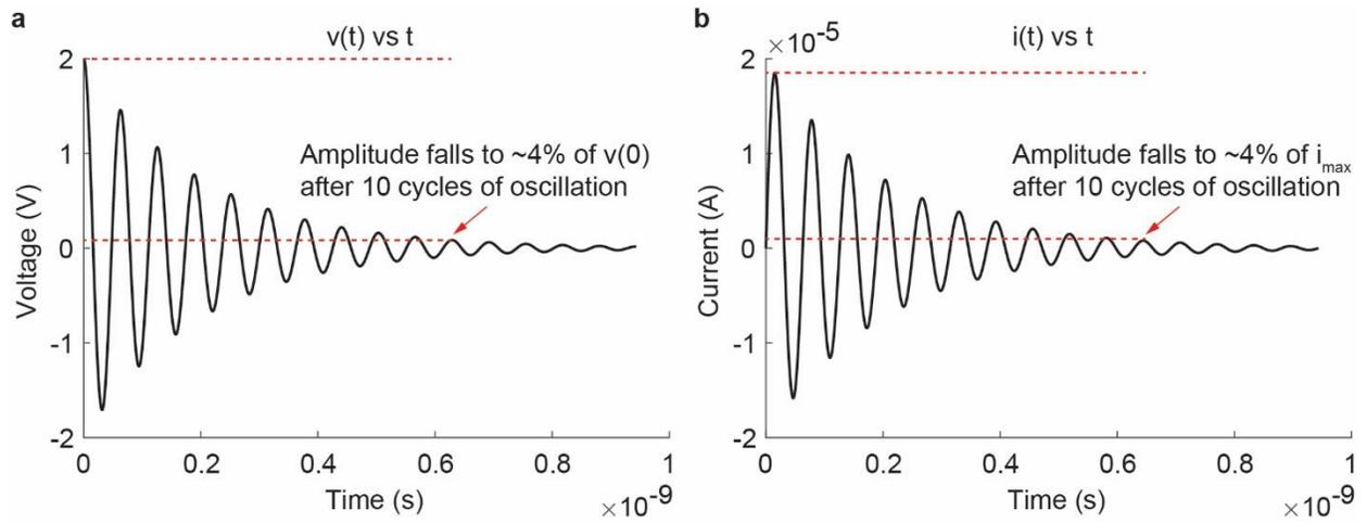
**Figure 2. Simulated  $v(t)$  and  $i(t)$  for a series RLC circuit with  $R = 10\text{k}\Omega$ ,  $L = 1\mu\text{H}$ , and  $C = 10\mu\text{F}$ .**
