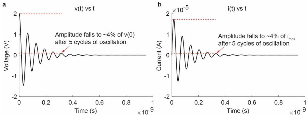
**Figure 1. Simulated  $v(t)$  and  $i(t)$  for a series RLC circuit with  $R = 20\text{k}\Omega$ ,  $L = 1\mu\text{H}$ , and  $C = 10\mu\text{F}$ .**
