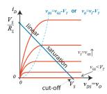
For proper operation, MOSFET must be biased in saturation.
