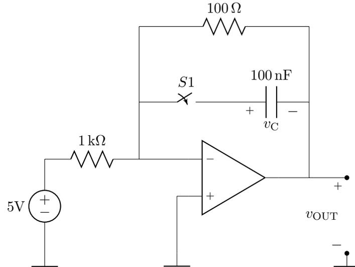
Consider the circuit shown above with switch S1 *initially open* and the source is a constant 5V. Assume that the Op-Amp is ideal.
