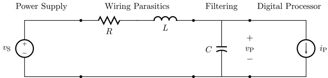
(2A) (5%) Derive a second-order differential equation that relates  $v_P$  to  $v_S$  and  $i_P$ .
